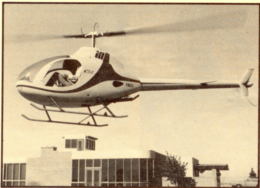
Fully enclosed doors (not shown here) are standard on the Exec, which has the same drive train and rotor system as the Scorpion, as well as a simplified cyclic system and lighter controls.
